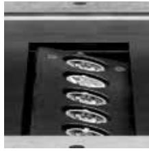
The LEDs are mounted on bars that are adjustable independently.
